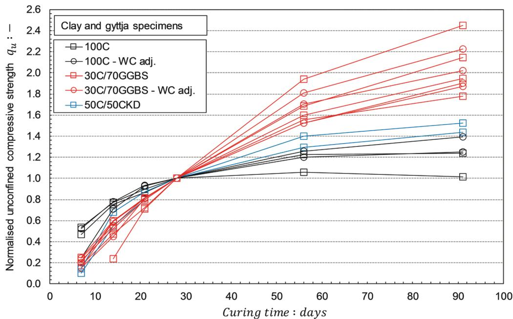
Fig. 7. Strength  $q_u$  normalised to strength at 28 days of curing vs. time.
